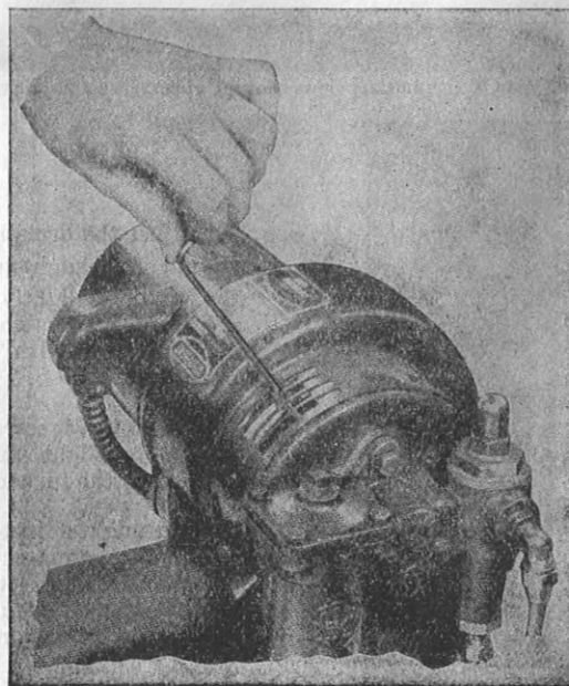
FIG. 12.—Removing pump. Loosen pump coupling by reaching through the air shutter with a long Allen wrench. Disconnect inlet and return line, if one be used, and the fuel line from the cut off valve to the nozzle line. Remove the two pump assembly mounting bolts and the pump can then be pulled straight out.
